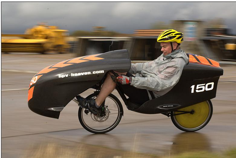
**Figure 2:** Recumbent cycle with front and rear fairings.
