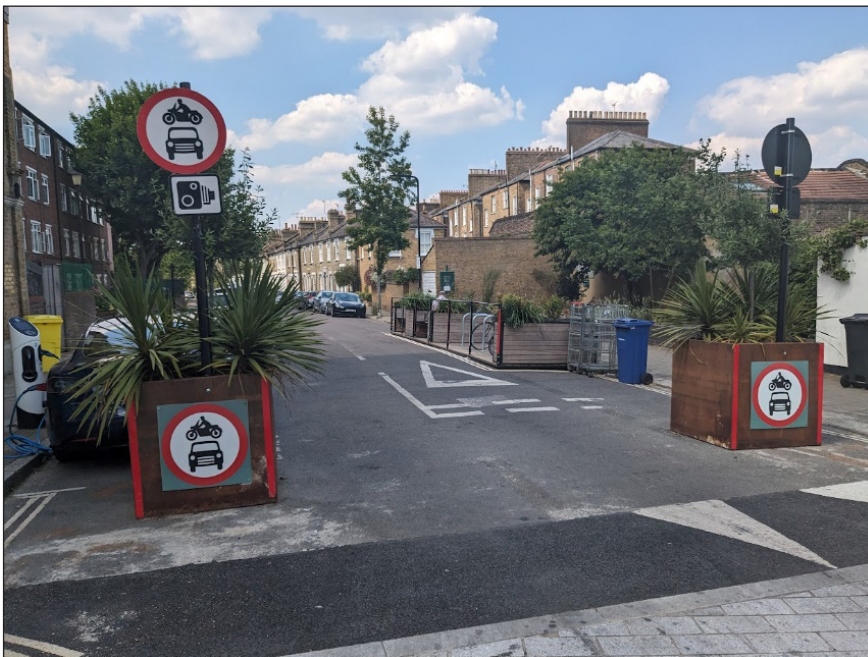
Figure 1: Automatic Number Plate Recognition (ANPR) enforced modal filter in a case study LTN. (A residential street where there are two planters on either side of the road with road signs that indicate there is no access for motor vehicles and that this is enforced using cameras.)
